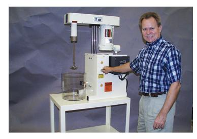
After 20 minutes, a sample from the batch should be checked for "fineness of grind" using a Hegman, Micron or NPIRI drawdown gauge.
